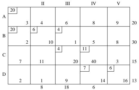
The cells which get allocation are called cells. Total transportation cost according to this allocation = 20(3) + 20(2) + 6(10) + 4(20) + 11940 + 7(14) + 6(16) = Rs. 878.**Example 2:**
