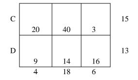
Next allocate  $x_{33} = Min [4, 15] = 20$  in the cell (3, 3). Requirements of III are satisfied. Score out the third column.
