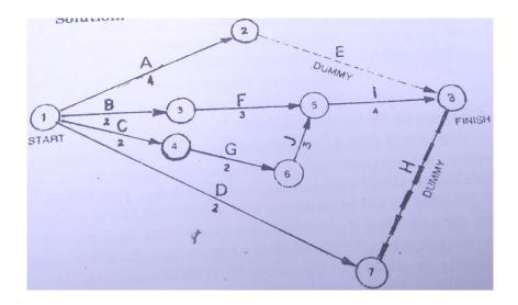
**Illustration 3**: From the following information draw up a Network diagram and indicate the Est, Lst, Eft and Lft of the various activities.
