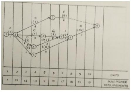
Figures indicated within the brackets above the arrow marks are the units of manpower required per day. The above diagram shows that the manpower requirements on various days do not remain within the constraint of 10 units of labour. Hence, it needs scheduling in the following manner:
