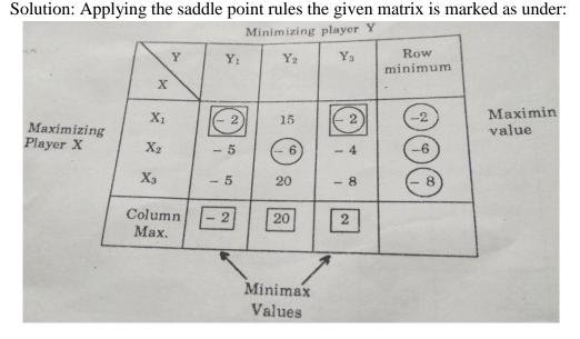
From the above marked matrix we find that there are two cells (1, 1) and (1, 3) that contain the element – 2 covered by both the mark  $\boxed{0}$  which is equal to both the maximum and minimax indicated therein. This shows that there are two saddle points in the given game viz., cell (1,1) and cell (1,3), where
